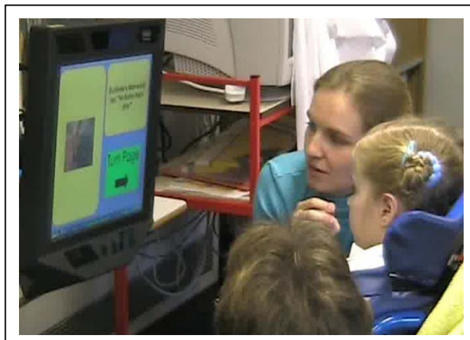
Figure 4.11. Helen is successfully reading a book and turning the page with her eyes, thanks to a combination of large targets and a special dwell-select feature that prevents her from being distracted by a pointer in her peripheral vision.
