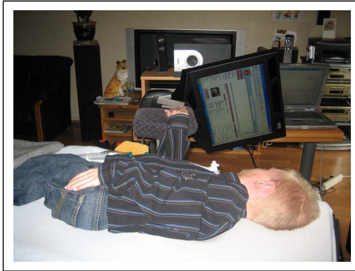
Figure 4.8. Bjorn Andre's eye-control is so good and his head is so still that he is able to have full control over all Windows applications, by using direct control of the on-screen pointer using his eyes, combined with a small on-screen keyboard.
