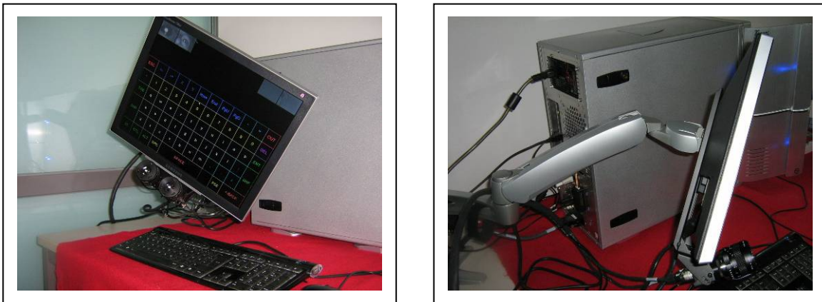
Figure 4.2. A fully adjustable Ergotron mounting arm, used here with the LC Binocular Eye Control System.
