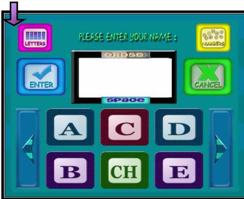
This window shows the letters from A to E that the user can use to create a user name. By using the arrows the user can access the next letters (f...k, l...p, q...v & w...z). The user can also go back to the general letters window (picture above) by entering the “letters” button or use the numbers (picture next page) by entering the “numbers” button.
