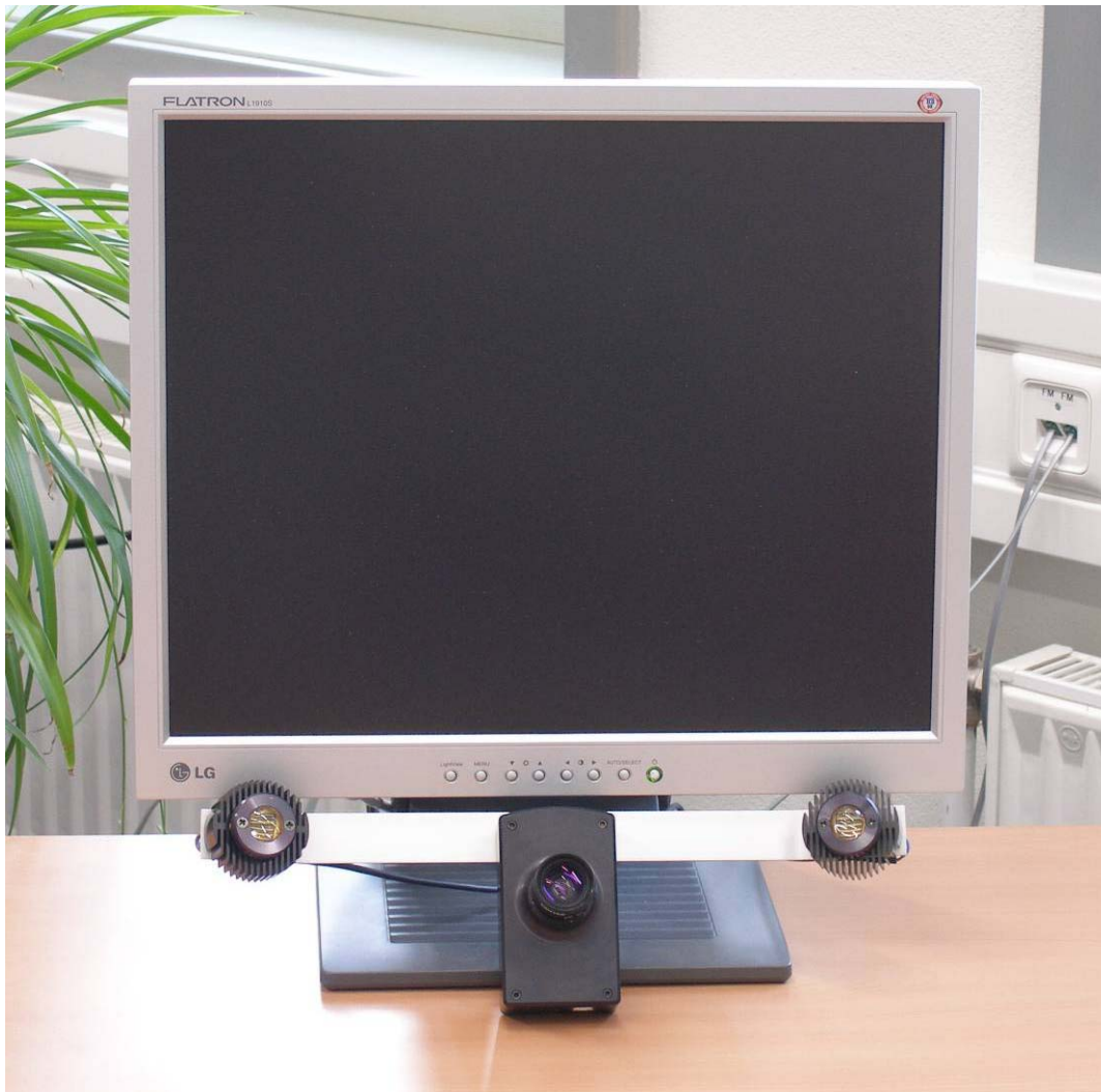
Figure 6.1: System setup of the remote eye tracker. The tracker consists of a single high-resolution camera and two infra-red light sources to either side of the camera, mounted below a computer display.
